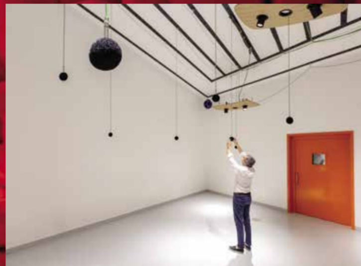
REV LAB, reverberation chamber
